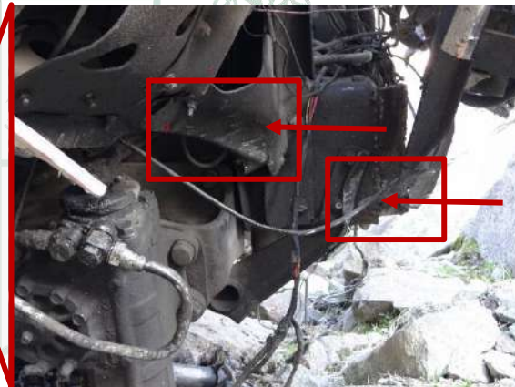
Metal marks of vehicle collision on right underside of bus
