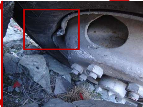
White car paint marks on the bus front right tire
