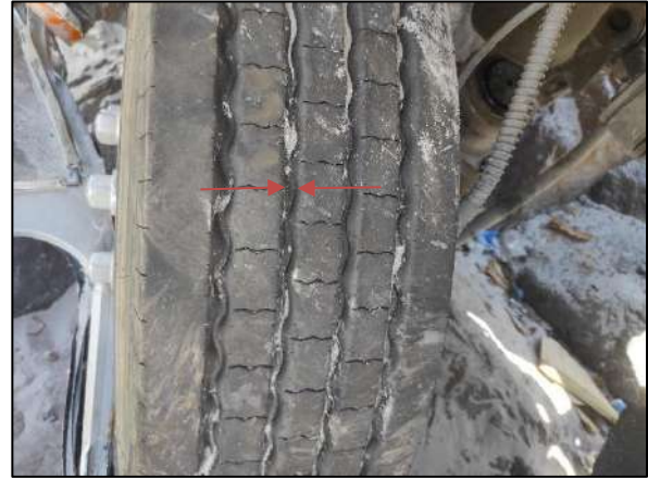
Tire Tread Acceptable Tread Depth
