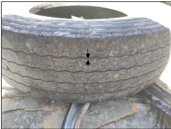
Tire Tread Acceptable Tread Depth
